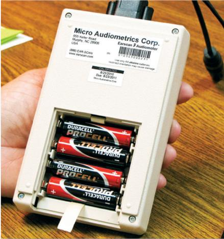
Insure proper orientation when installing batteries.
