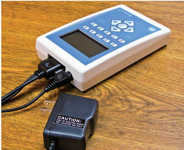
When using AC power, use only the supplied adapter. To power from a PC use the supplied USB cable.
